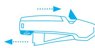
Slide the lock to the rear position, so that the **lever can be released** again. **Then** push the blade change button back into the handle and continue cutting.
