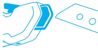
Now **reverse or change** the blade. Make sure that the blade is exactly positioned on the cams on the blade holder.
