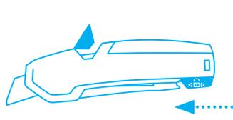
Secure the lever with the safety device and turn the handle so that the **transparent blade cover is facing upwards**.
